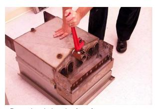
Removing drain valve from frypot.
